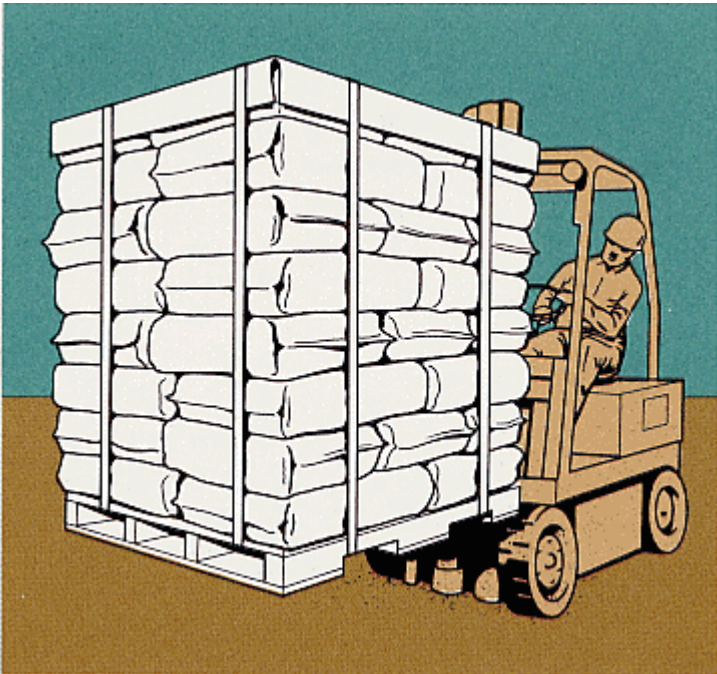
Palletized Load of Bagged Cargo
